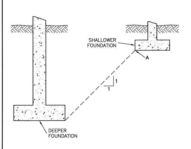
NOTE: POINT "A" OF SHALLOWER FOOTING MUST BE SITUATED BELOW THE DASHED LINE SHOWING THE FOOTING LOCATION LIMIT.
