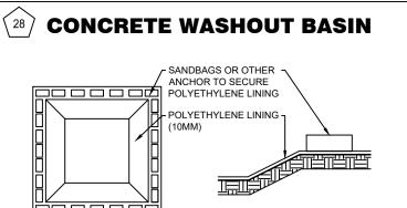
INSPECT WEEKLY AND AS DIRECTED IN THE STORMWATER POLLUTION PREVENTION PLAN, REPAIR/REPLACE AS NEEDED REMOVE COLLECTED CONCRETE WHEN THE APPEARS 1/3 FULL DISPOSE OF INORGANIC MATERIAL PROPERLY.
