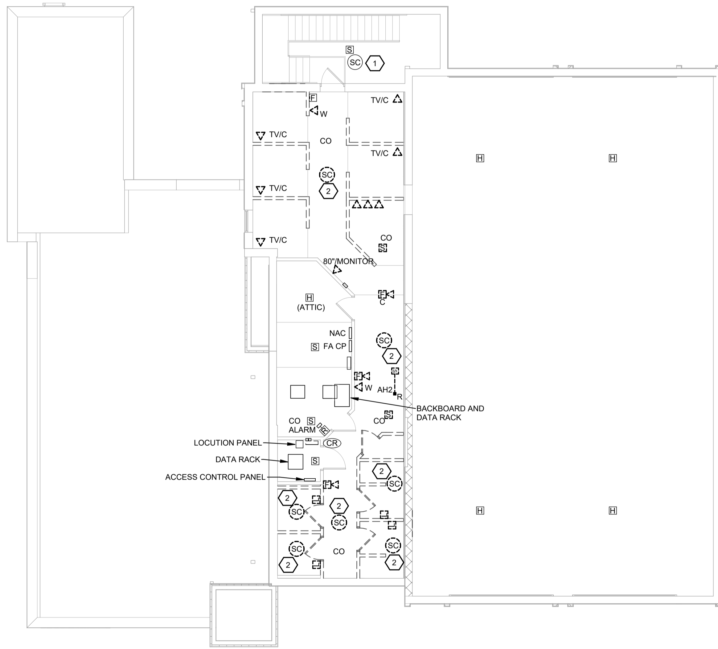
SECOND FLOOR DEMOLITION PLAN - SYSTEMS - PHASE 2 SCALE: 1/8" = 1'-0"
