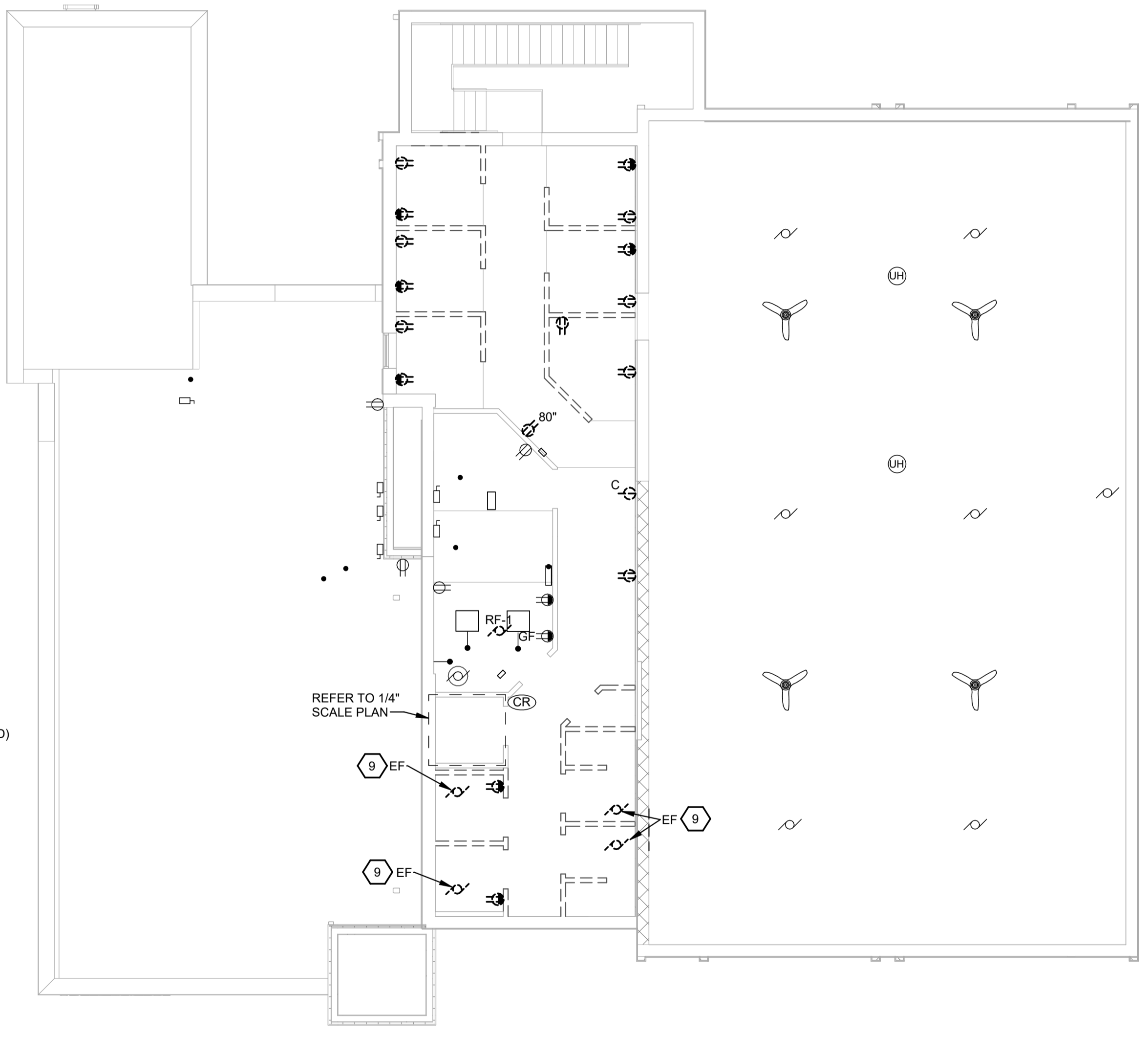
SECOND FLOOR DEMOLITION PLAN - POWER - PHASE 2 SCALE: 1/8" = 1'-0"
