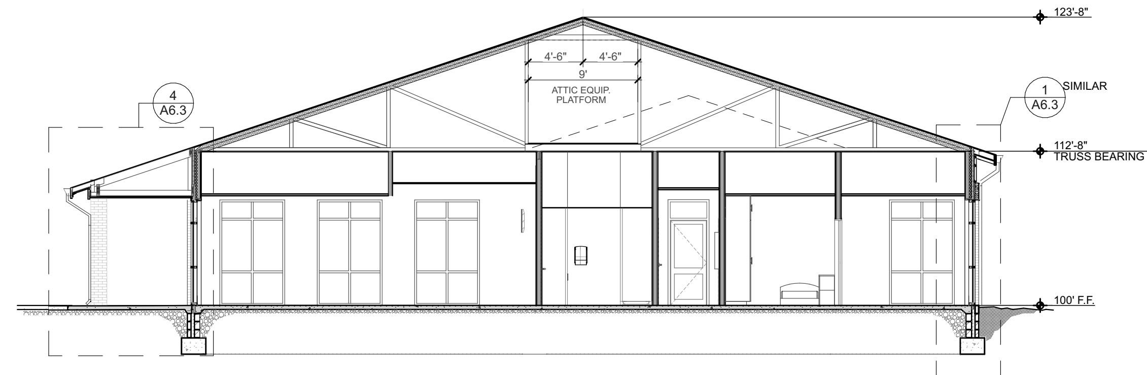
2 BUILDING SECTION SCALE: 1/8" = 1'-0"
