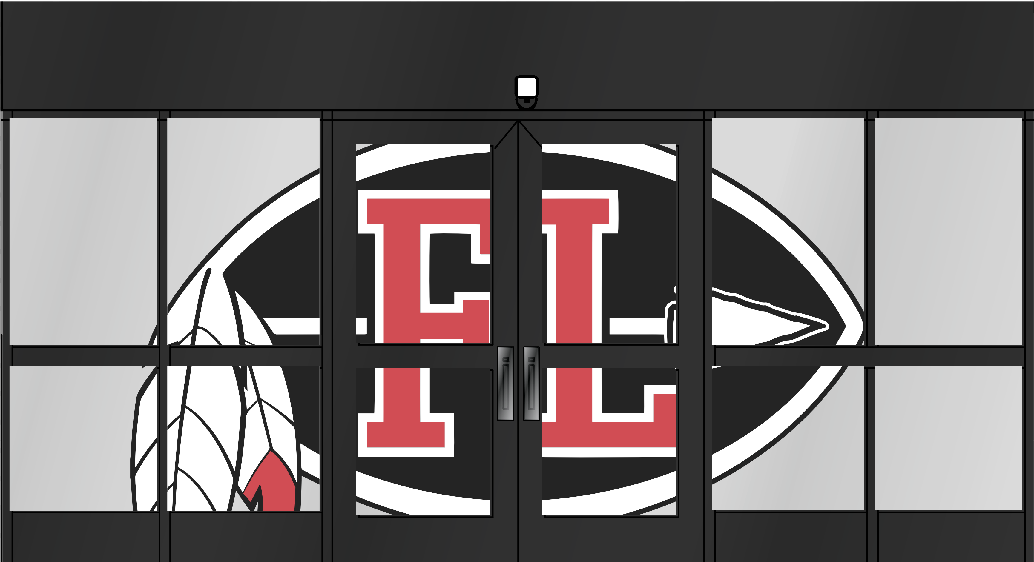
WINDOW VINYL - DETAIL 80/20 WINDOW PERF, ADHESIVE BACKING
