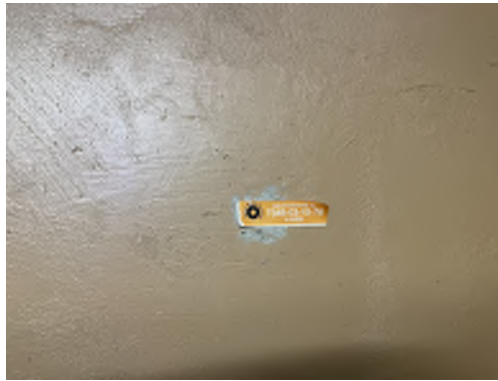
Sample 7348-03-10-76 with no detectable lead
