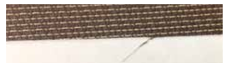
Fiberglass fabric with Fraying
