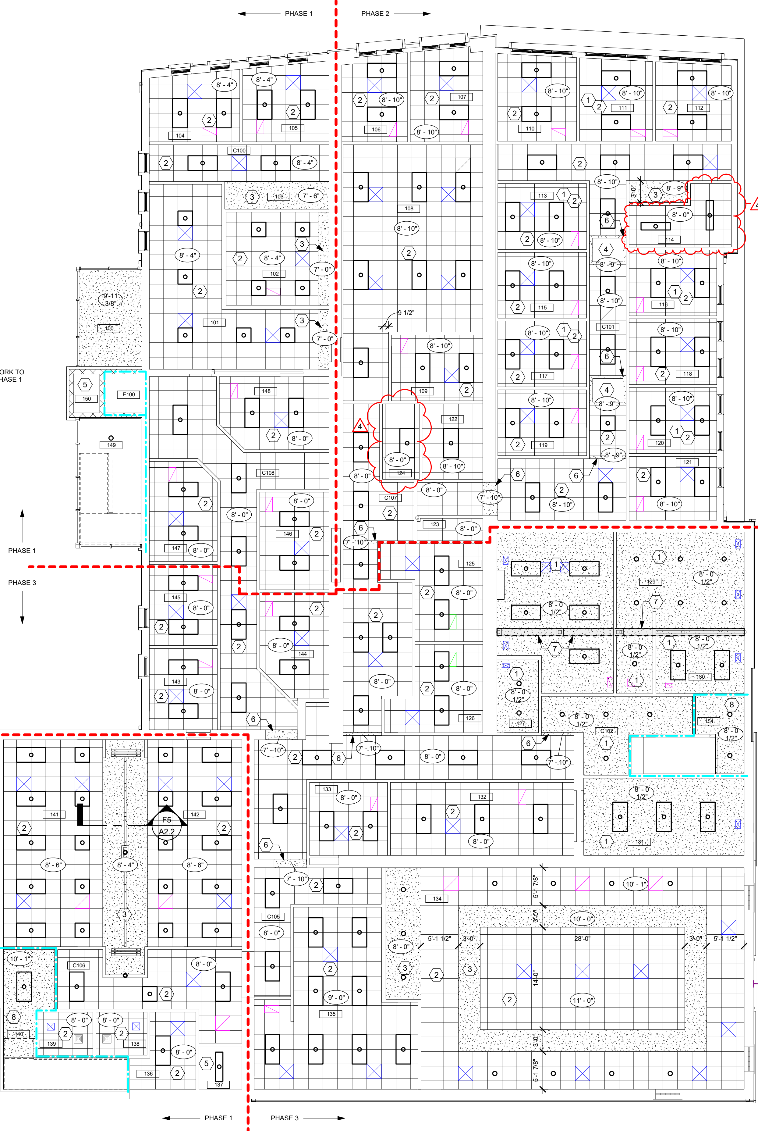
(F2) FIRST FLOOR NEW WORK REFLECTED CEILING PLAN 1/8" = 1'-0"
