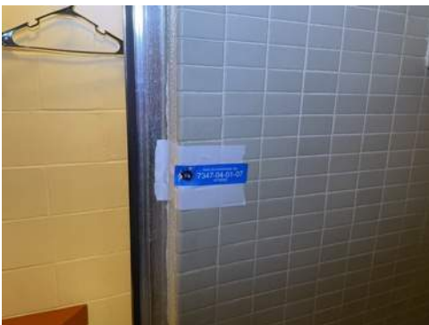
Photo 43- Sample# 7347-04-01-07, No Asbestos Detected in Ceramic Tile, Tan Adhesive, and Grout
