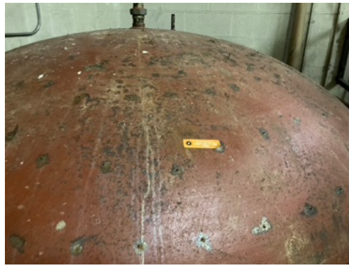
Paint Film Sample 7347-03-11-62 with 0.648% lead
