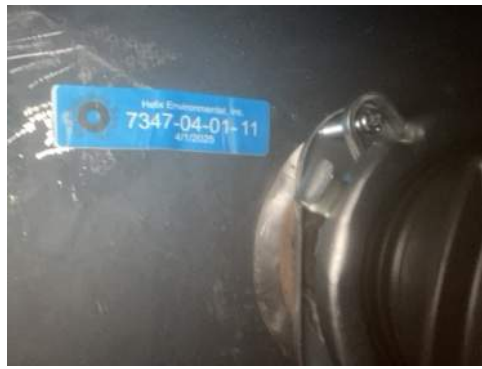
Photo 47- Sample# 7347-04-01-11, No Asbestos Detected in Sink Soundproofing
