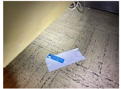
Photo 21- Sample# 7347-03-11-21, 0.6% Chrysotile Asbestos Detected in 12"x12" Grey Streaked Floor Tile, No Asbestos in Black Mastic
