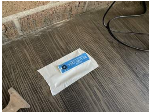
Photo 08- Sample# 7347-03-11-08, No Asbestos Detected in Sheet Flooring and Green Mastic
