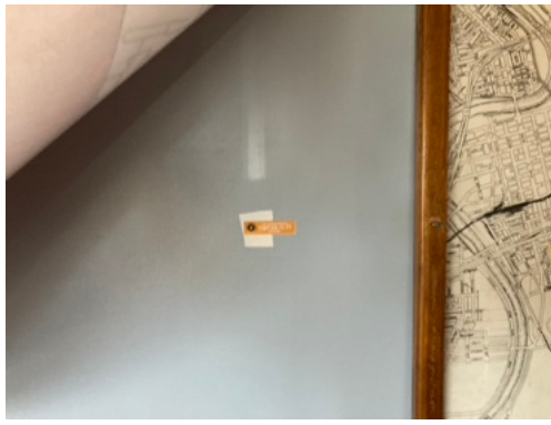
Paint Film Sample 7347-03-11-71 with no detectable lead
