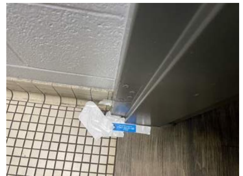
Photo 45- Sample# 7347-04-01-09, No Asbestos Detected in Ceramic Tile, Tan Adhesive, and Grout
