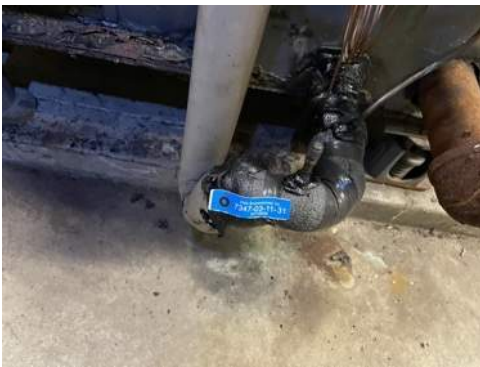
Photo 31- Sample# 7347-03-11-31, No Asbestos Detected in Black Sweat Wrap
