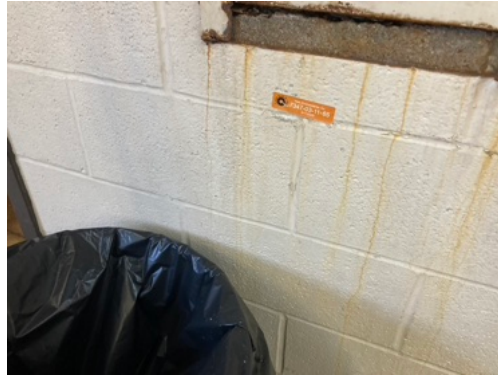
Paint Film Sample 7347-03-11-65 with no detectable lead
