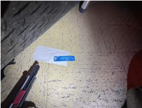
Photo 22- Sample# 7347-03-11-21, 0.4% Chrysotile Asbestos Detected in 12"x12" Grey Streaked Floor Tile, No Asbestos in Black Mastic
