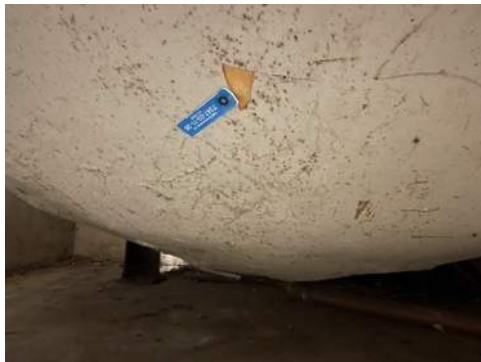
Photo 26- Sample# 7347-03-11-26, 10% Chrysotile Asbestos Detected in Grey Tank Insulation Sealant
