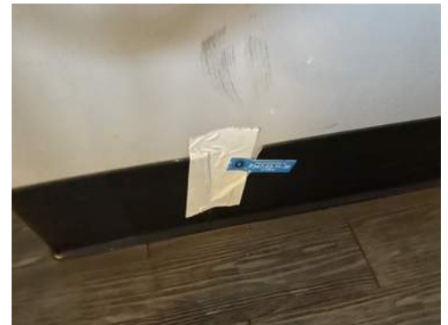
Photo 36- Sample# 7347-03-11-36, No Asbestos Detected in 6" Cove Base and Mastic
