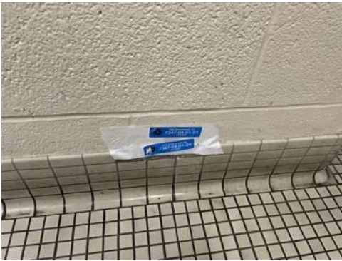
Photo 40- Sample# 7347-04-01-05, No Asbestos Detected in Ceramic Tile, Tan Adhesive, and Grout
