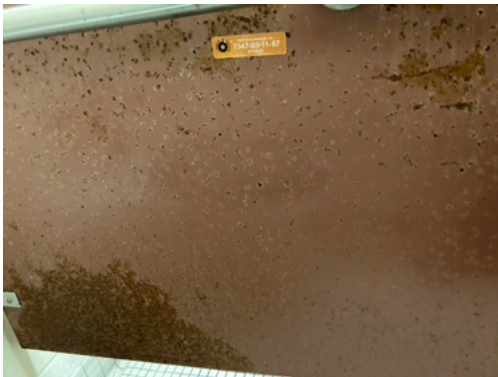
Paint Film Sample 7347-03-11-67 with 1.049% lead
