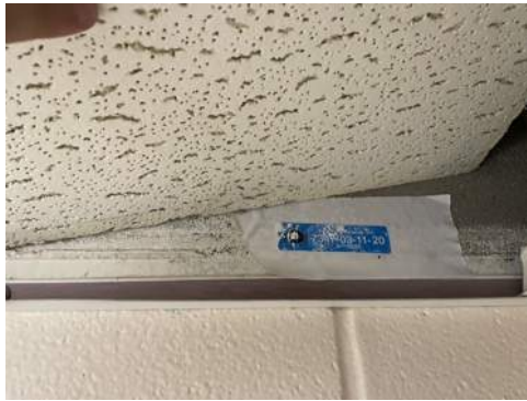
Photo 20- Sample# 7347-03-11-20, No Asbestos Detected in Stucco
