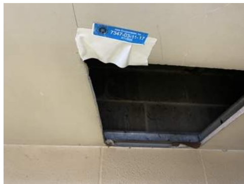
Photo 17- Sample# 7347-03-11-17, No Asbestos Detected in Drywall and Joint Compound
