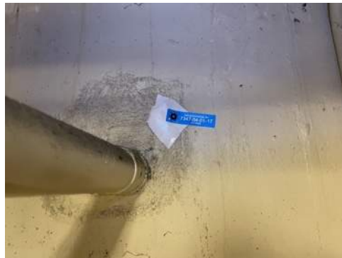
Photo 53- Sample# 7347-04-01-17, No Asbestos Detected in Pipe Penetration Mortar
