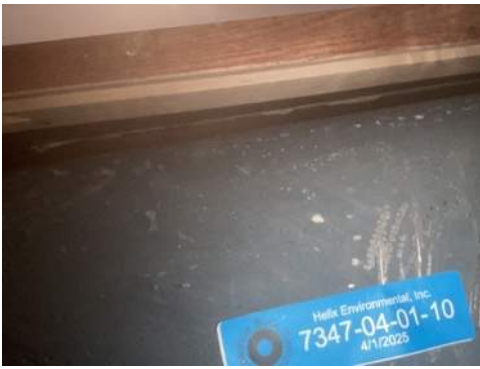
Photo 46- Sample# 7347-04-01-10, No Asbestos Detected in Sink Soundproofing
