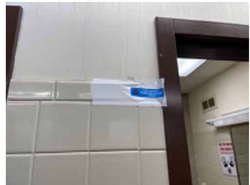
Photo 63- Sample# 7348-03-31-09, No Asbestos Detected in Tan Ceramic Tile Adhesive
