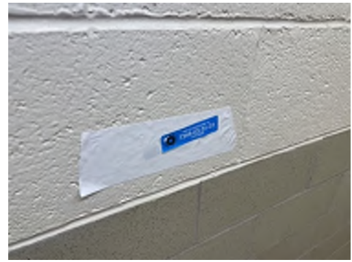
Photo 57- Sample# 7348-03-31-03, No Asbestos Detected in Yellow Block Coating
