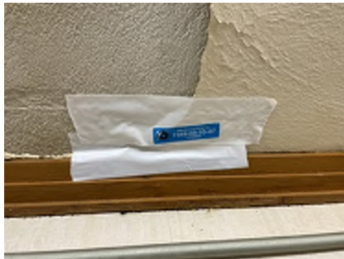
Photo 47- Sample# 7348-03-10-47, No Asbestos Detected in Hard Plaster and Skim Coat
