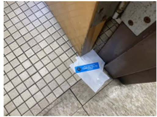
Photo 66- Sample# 7348-03-31-12, <0.25% Asbestos Detected in Mortar, No Asbestos Detected in Ceramic Tile and Adhesive
