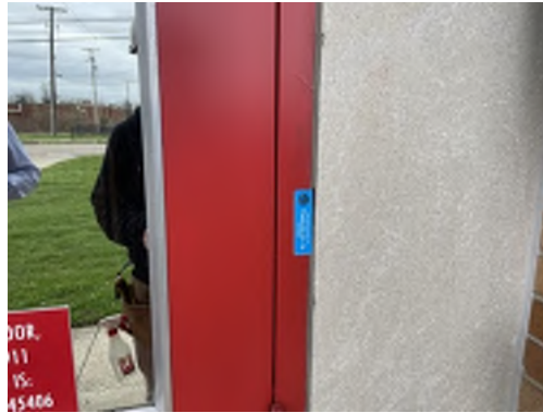
Photo 68- Sample# 7348-03-31-14, No Asbestos Detected in Grey Exterior Caulk
