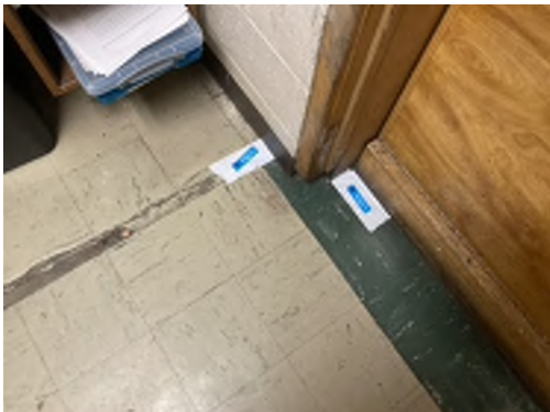
Photo 34- Sample# 7348-03-10-34, 4% Asbestos Detected in 9"x9" Green Streaked Floor Tile, No Asbestos in Black Mastic
