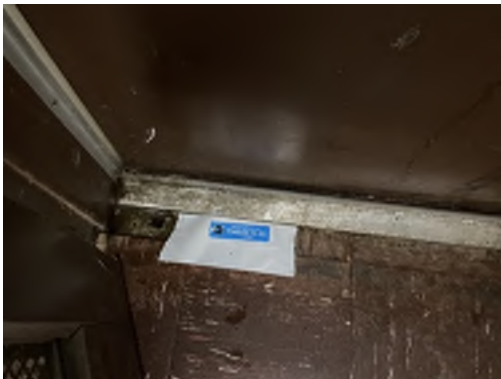
Photo 43- Sample# 7348-03-10-43, 1.3% Asbestos Detected in 9"x9" Maroon Streaked Floor Tile, No Asbestos in Black Mastic
