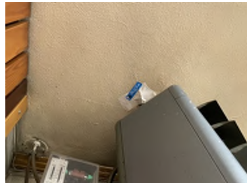
Photo 48- Sample# 7348-03-10-48, No Asbestos Detected in Hard Plaster and Skim Coat
