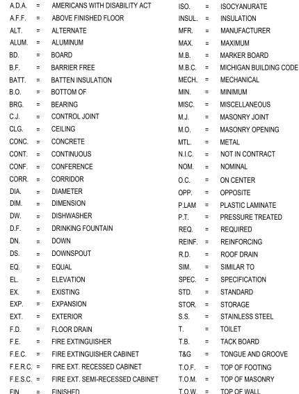
T.O.W. = TOP OF WALL FIN. = FINISHED TYP. = TYPICAL FLR. = FLOOR U.N.O. = UNLESS NOTED OTHERWISE F.R.T. = FIRE RETARDANT TREATED V.I.F. = VERIFY IN FIELD GA. = GAUGE
