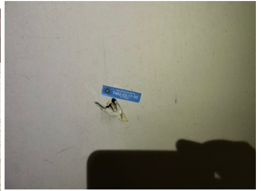
Photo 39 - Sample 7462-03-17-50, 4% Asbestos Detected in Joint Compound only
