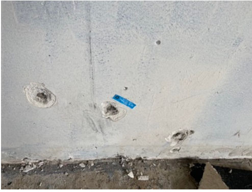
Photo 82 - Sample 7462-03-18-35, No Asbestos
