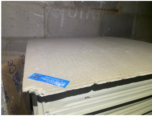
Photo 105 - Sample 7462-03-31-12 with no detectable asbestos
