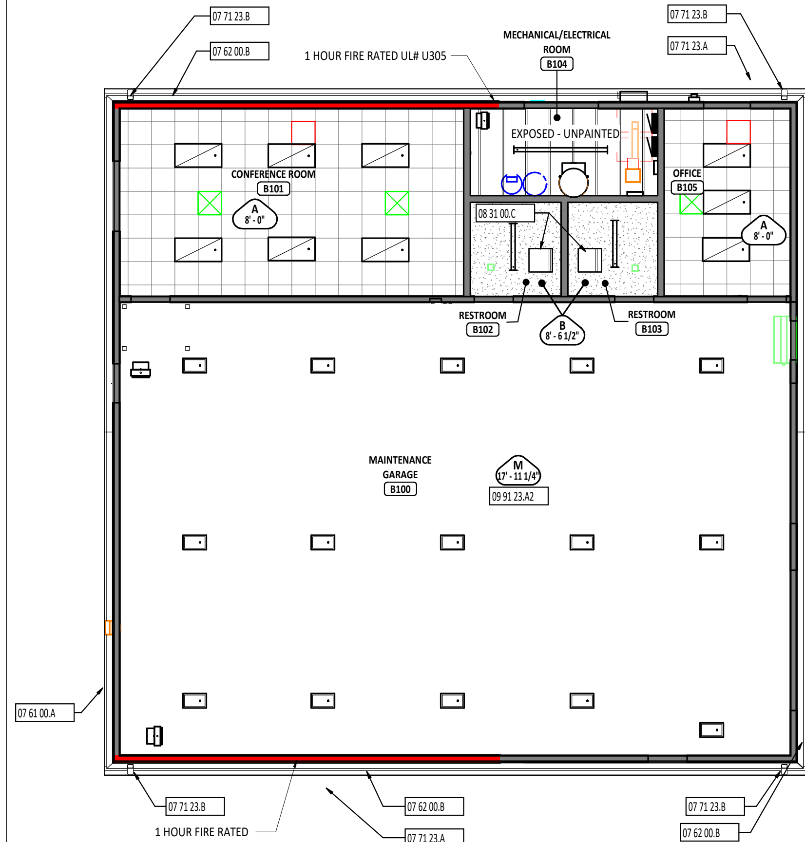
4 FIRST FLOOR REFLECTED CEILING PLAN - UNIT B 1/8" = 1'-0"
